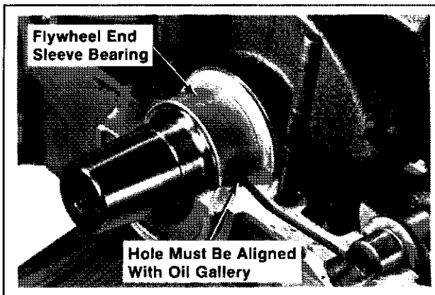
Figure 11-13. Position of Flywheel Bearing.
